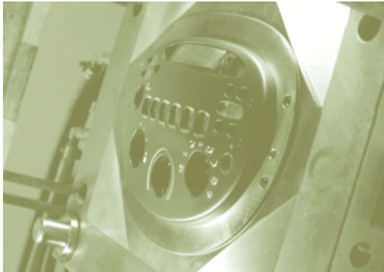
The decorated, formed film is positioned in the mold and then backfilled with transparent polycarbonate.
